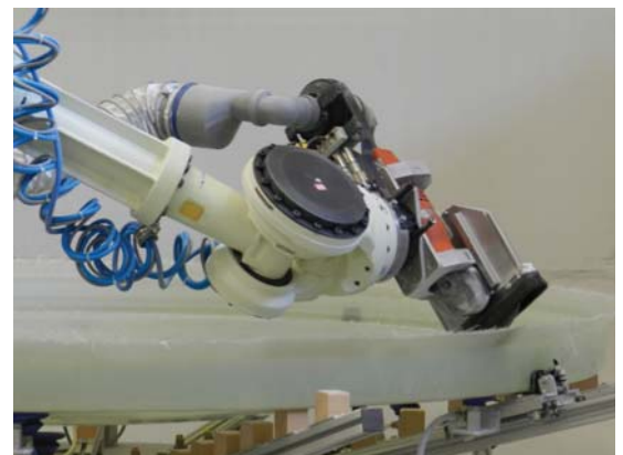
The Kawasaki ZT130L working the edge of a tank bottom.
