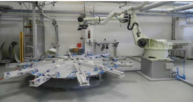
The Kawasaki ZT130L robot has been combined with an automatic tool change system and specially developed rotary tables.
