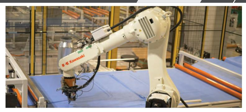
Once the tabletop workspace is covered in material, the robot uses a tool changing station to equip a proprietary rotary ultrasonic welding horn designed by Harbour Technologies. Using this tool, the robot traces the gown profile to bond the front and back pieces of material together.
