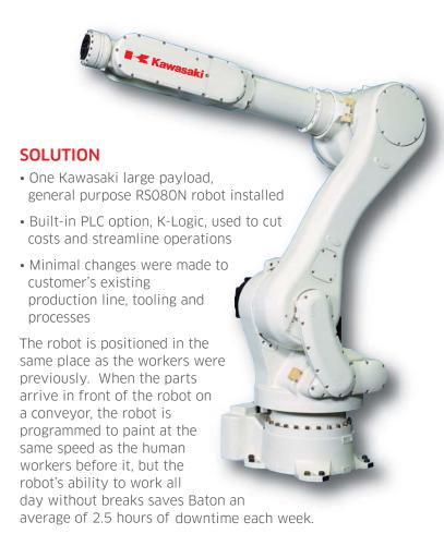
Choosing a robot from Kawasaki's line of high performance general purpose robots, as opposed to paint robots, was a purposeful choice by the integrator, who picked this specific model due to its long reach capabilities. The RS080N robot's extended reach (2,100 mm) made it perfect for Baton's application, which required the robot to spray a large area from one fixed location.
